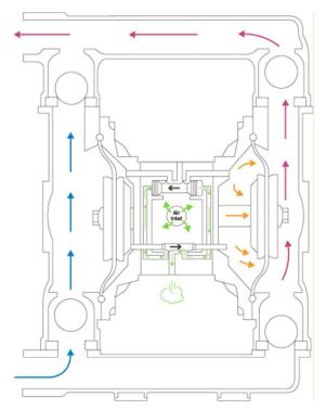
With air turned on, piston pushes to one side to start Drawing in the liquid Pushing the liquid out
