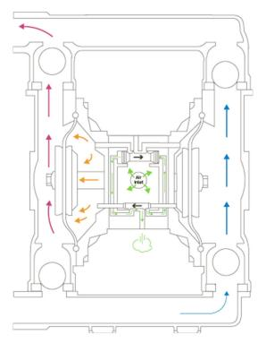
Then alternating back Drawing in the liquid Pushing the liquid out
